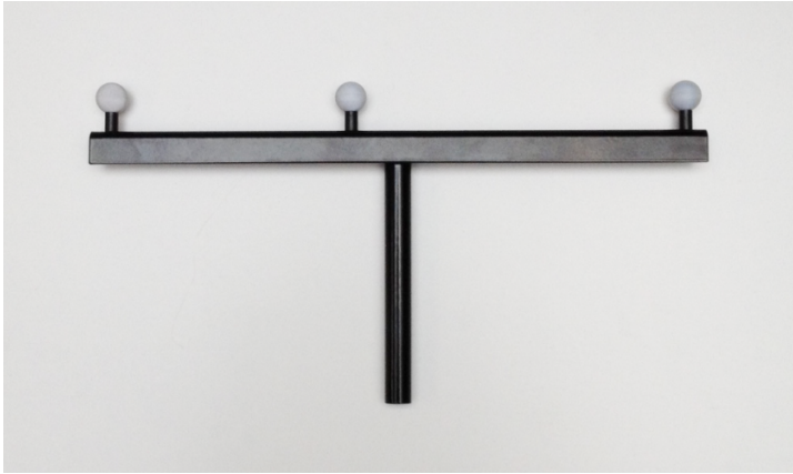
Figure 7.14: Registration device used for setting up multiple PST units
